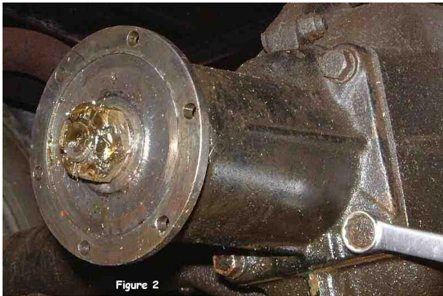
With the carrier up on the bench, remove the cotter pin from the pinion nut and discard the cotter pin. The pinion nut may be very tight. Clamping the flange across the edges in a vise is a good way of holding the pinion from turning. That is a  $\frac{3}{4}$ " drive socket being used to loosen the nut as shown in Figure 3.
