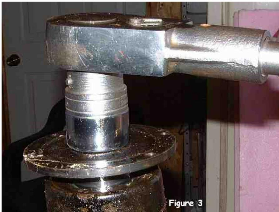
Once the nut is loose, turn the nut off until it is flush with the top of the pinion. Leave the nut on to protect the top of the threaded pinion shaft when you use the puller to remove the flange in the next step. See Figure 4 below. The flange maybe fairly tight and will require a good two jaw or even better, a three jaw puller. As the flange is drawn up the shaft, turn the nut up and off as required until you can tap the flange off with a soft hammer.
