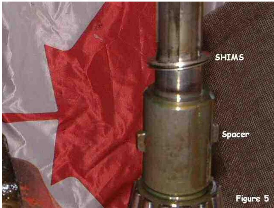
By using a long punch on the inner race of the outer bearing, the bearing and seal can be driven out the front of the carrier. Or, use a pry bar and try to lever the old seal out. It will be tight and difficult to pry. Now is the time to wash all the components to check for any problems with them. Examine bearings, cups and cones. If the cups show signs of bad wear or if time has broken through the hard cup surface, the bearing should be replaced. Now is the time to do it!!!
