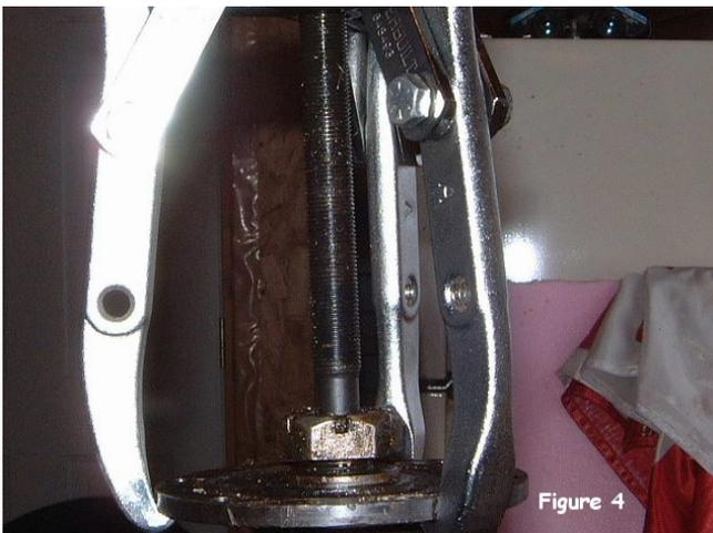
Once the nut is loose, turn the nut off until it is flush with the top of the pinion. Leave the nut on to protect the top of the threaded pinion shaft when you use the puller to remove the flange in the next step. See Figure 4. The flange maybe fairly tight and will require a good two jaw or even better, a three jaw puller. As the flange is drawn up the shaft, turn the nut up and off as required until you can tap the flange off with a soft hammer.
