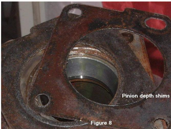
When replacing the assembly, clean the mating surfaces and be sure you replace the original two gaskets and shim. See Figure 8. They determine the depth of the pinion to the ring gear and must be correct!!! Coat the threads on the housing cap screws with sealer and tighten them gradually using a criss-cross pattern. Replace the drive shaft using your original marks as a guide. Check the oil level in the differential, top up if necessary.
